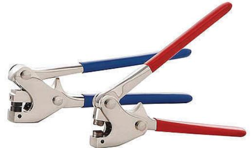
Alpha numeric characters can be engraved onto the dies on request. The characters are then transferred to the seal when it is compressed and identify which set of pliers (and so which operator) carried out the sealing operation.
