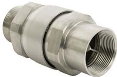
These couplings will separate when a pre-determined force is applied in an angular direction up to 45° from the axis of the coupling. The separation is a clean and dry break, keeping spillage to a minimum, and they are repairable (with one set of spare shear pins being carried on-board each unit). Seals are suitable for aviation jet fuels.
